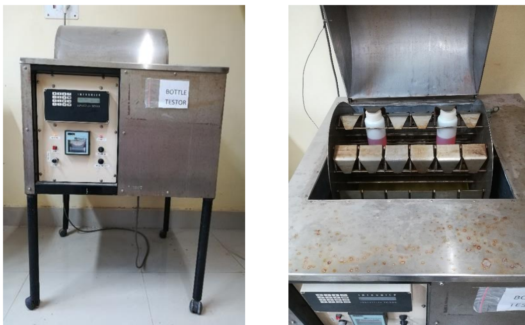
Figure 1. Water bath used for test work.
